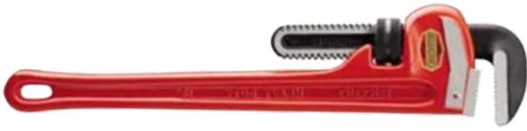
Ridgid Brand, 14" Iron Pipe Wrench, 2" Pipe Capacity, Straight Sturdy Cast Iron Housing, I-Beam Handle, Full Floating Hook Jaw With Spring Suspension, Replaceable Jaws With Tough, Heat Treated High-Alloy Steel Jaw Teeth, Extra Strong Mount For Heel Jaw.
