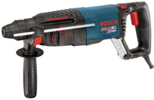
This powerful hammer delivers 2 ft.-lbs. of impact energy and 0-5,800 no-load BPM, but it weighs just 6.7 lbs. The multifunction mode selector allows users to easily select among three modes of operation: rotary hammer, rotation only and hammer only. To optimize the chiseling angle, it has Vario-Lock positioning that rotates and locks the chisel in one of 36 different positions.
